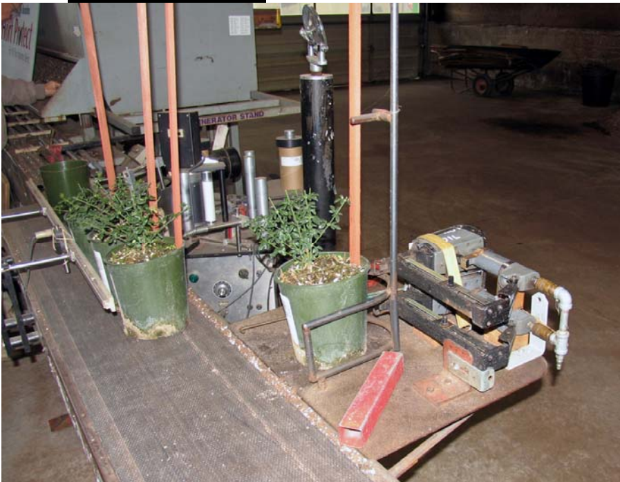
Above: An automatic staple machine to staple the sticks onto a pot for clematis. This process was stated to be "faster and safer".
